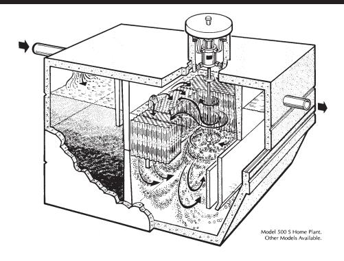
The compact, efficient BIOLOGICALLY ACCELERATED TREATMENT™ Plant – which we call the JET BAT® Plant – has three compartments. The Pretreatment Compartment, on the left, receives the wastewater and partially treats it physically and biologically before it enters the Center Treatment Compartment.
