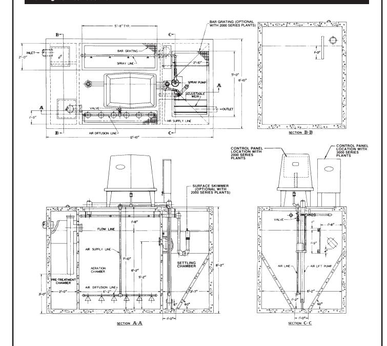
Note: To minimize fall thru plant, locate inlet invert 6" above flow line.
